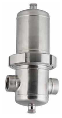
In process industries where the risk of corrosion of the compressed air system components is high, Pneumatech's FP 1-18 process filter range provides the right solution. The filter housing is made out of stainless steel grade 1,4301. The surface has been smoothened with advanced mechanical and electro-polishing techniques to a level of Ra 1,6. To avoid
